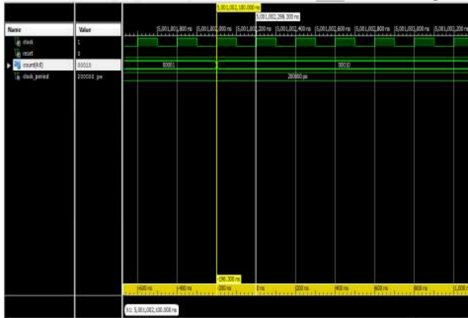
Figure 4: Test bench Behavioural for counter 5-bit
